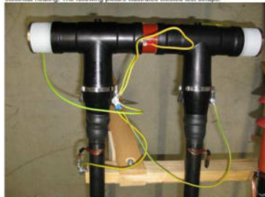
Figure 2: Two test objects of CTS-S with voltage sensor coupled with bushing (Euromet)
