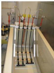
Figure 5: Electrical heat cycling in air
